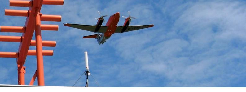
FCS employs Learjet or optionally King Air 350 aircraft for radar flight testing. FCS also provides SASS-C or equivalent ground recording and evaluation systems for documentation of compliance with applicable ICAO Doc 8071 and EUROCONTROL surveillance standards.
